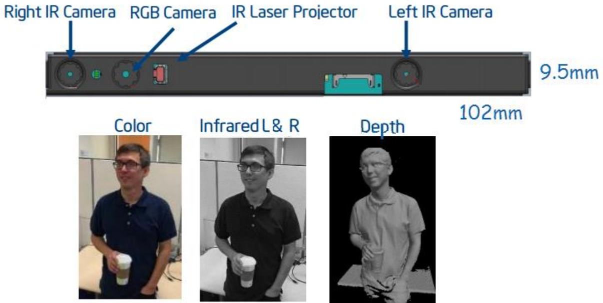
FIGURE 1: A breakdown of the RealSense camera and the images it can produce. Photo provided by Intel© Developer Zone.
