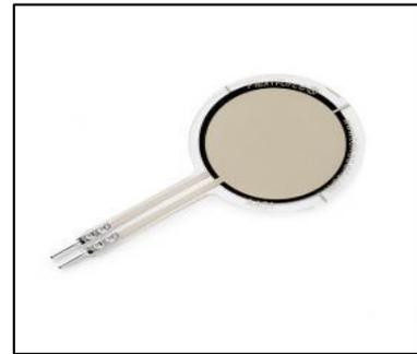
*Figure 3 Force Sensitive Resistor*
