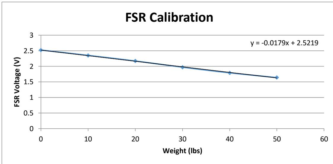
Figure 4 Force Sensitive Resistor
