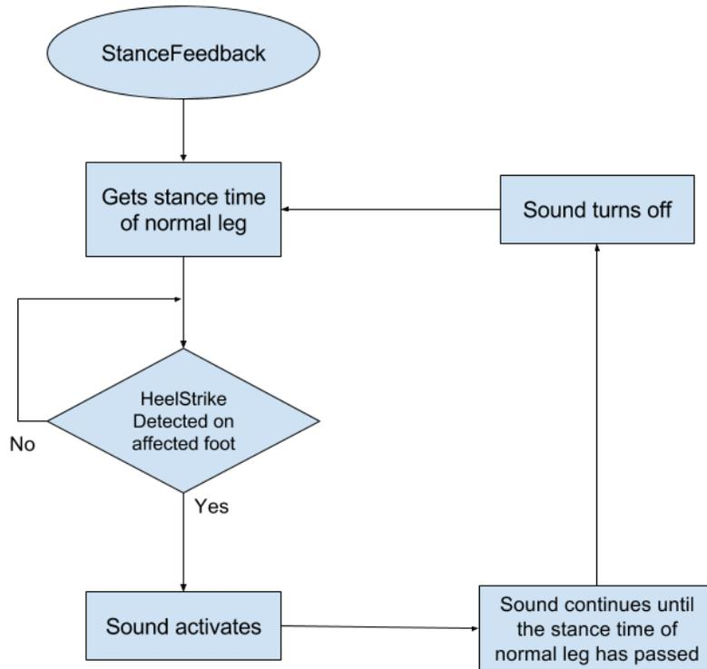
Figure 10 Flowchart for Stance Feedback
