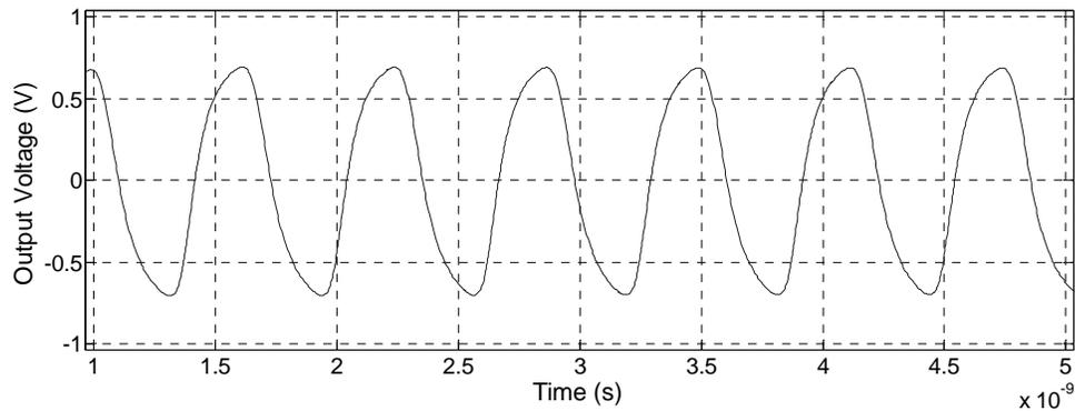
Figure 14. CML Buffer S6 Output Voltage at the SS Corner
