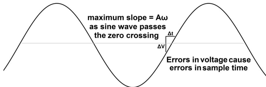
Figure 3. Sine Wave Illustrating Need for High Edge-Rates
