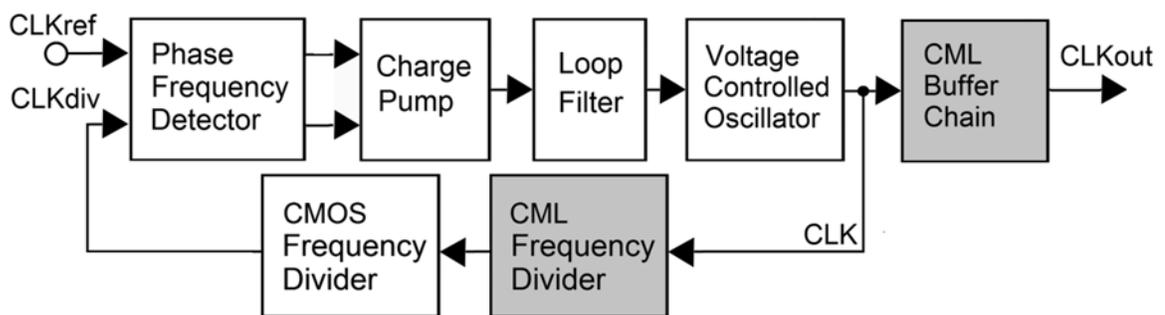
Figure 1. Phase-Locked Loop Block Diagram
