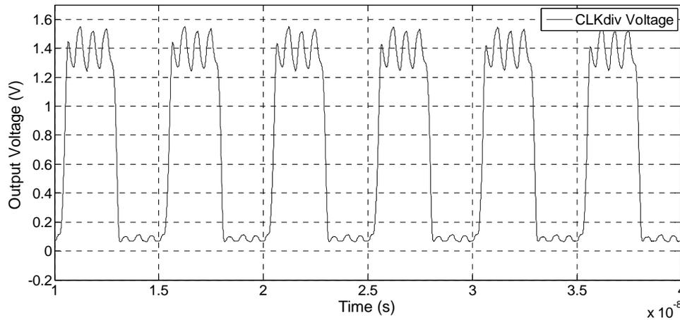
Figure 18. CML-to-CMOS Converter Output Voltage at the SS Corner with Noise
