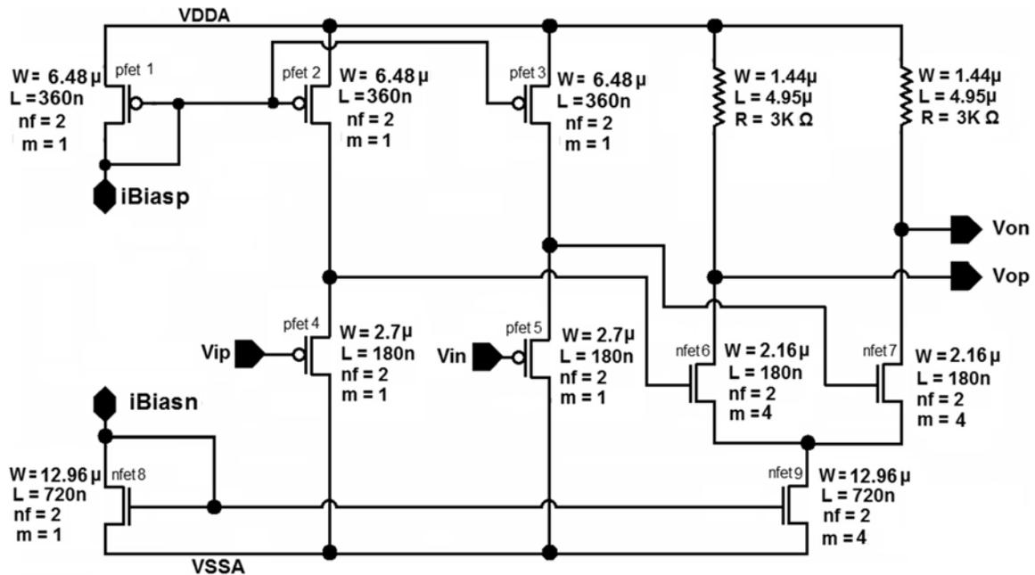
Figure 5. P-to-N Converter
