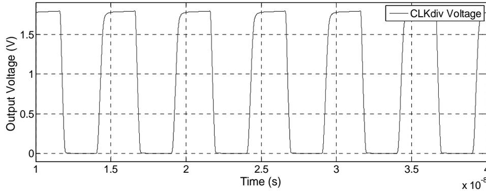
Figure 17. CML-to-CMOS Converter Output Voltage at the SS Corner without Noise
