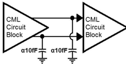
Figure 11. Added Parasitic Capacitance
