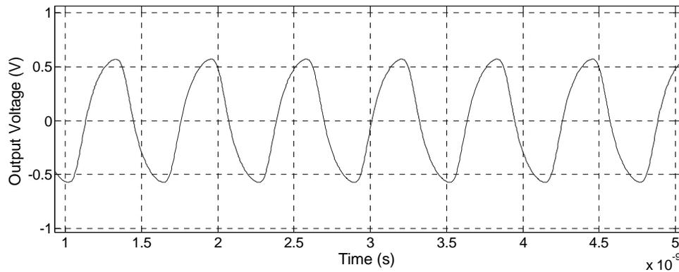
Figure 13. CML Buffer S1 Output Voltage at the SS Corner
