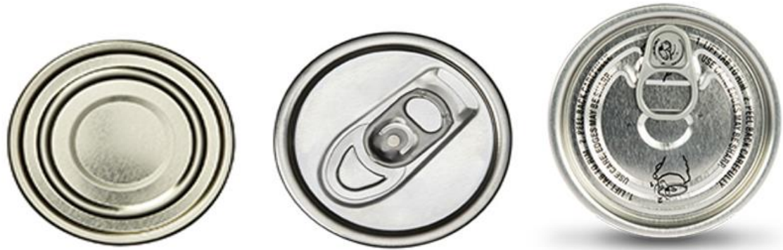
Figure 1. Examples of three different styles of ends. From left to right, the styles are sanitary end, a Stay-On-Tab (SOT) beverage end, and a Full-Panel, Pull-Open (FPPO) end.
