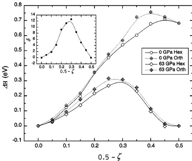
FIG. 4. Enthalpy changes along the orthorhombic and the monoclinic paths to rocksalt at 0 and 63 GPa. The inset shows the deviation from the ideal orthorhombic structure, in which  $\delta = (g_{13} + g_{23} - g_{33})/g_{33}$  (in %). For the orthorhombic structure,  $\delta = 0$ .
