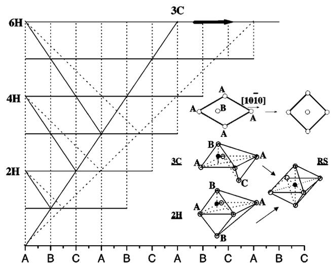
FIG. 1. Stacking sequence in hexagonal and cubic polytypes and their transformation through a layer shuffle movement to rocksalt. The top inset show the in-plane  $\gamma$  shear. The bottom inset shows how adjacent tetrahedra join into an octahedron for 3C and 2H. Open (closed) spheres are Si (C).
