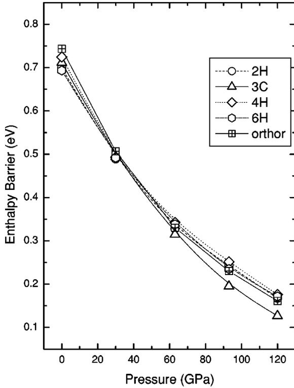
FIG. 3. Enthalpy barriers of the transitions to RS for the SiC polytypes as function of pressure.
