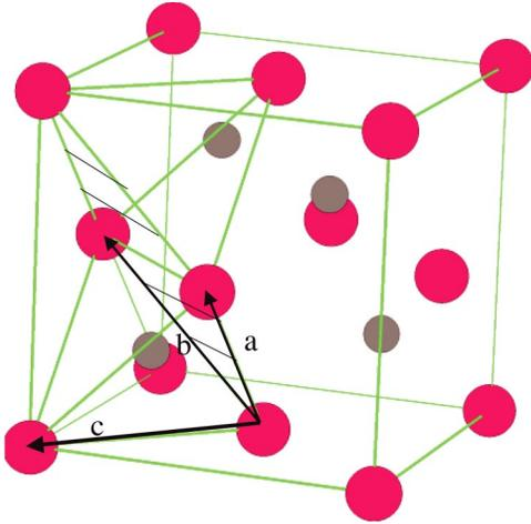
FIG. 2. Relation between the monoclinic intermediate state unit cell and the conventional cubic unit cell of 3C. See text.
