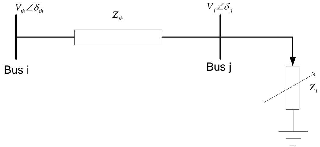
Figure 3.4: Equivalent circuit of Figure 3.3
