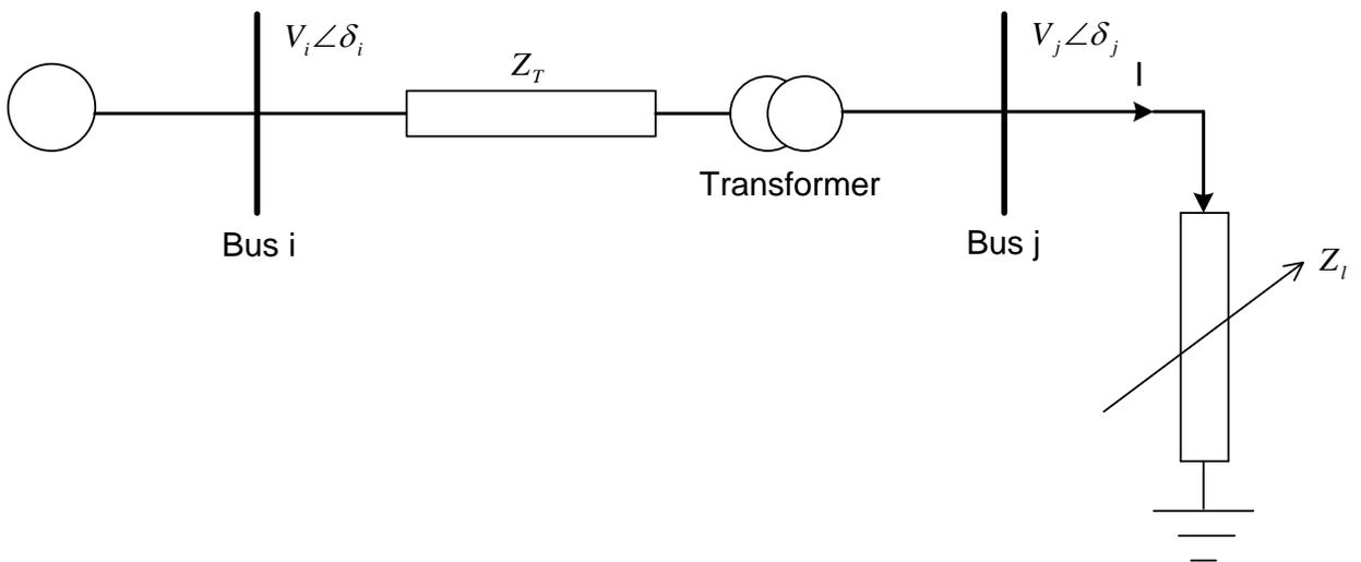
Figure 3.2 Simple two-bus system with transformer having off nominal turns ratios
