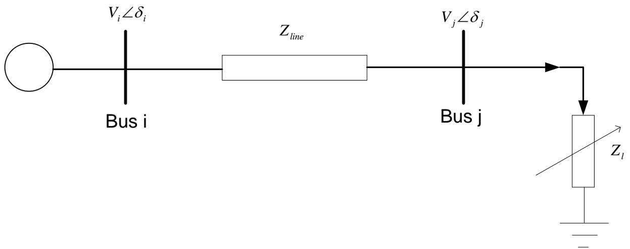
Fig 3.1 Simple two bus system to determine LVSI
