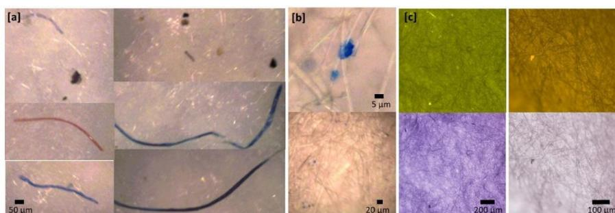
Figure 8. Representative photographs of different contaminants. Select fibers and fragments filtered out of “raw” (i.e., not doubly filtered) (a) Milli-Q deionized water, (b) one cluster of secondary contamination encountered on a Nile red stained filter, and (c) fluorescent (top) and visual (bottom) pictures of a GF filters dyed with Nile red.
