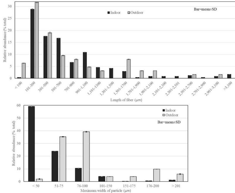
Figure 2. Size distribution for all fibers (top) and fragments (bottom) counted and measured on sample GF filters. Bins are  $25 \mu\text{m}$  for fragments and  $200 \mu\text{m}$  for fibers (due to the greater range of sizes). Bars: mean  $\pm$  1SD.
