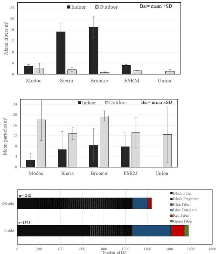
Figure 3. Microplastic fiber (top) and fragment (middle) counts per m<sup>3</sup> of air sampled across CSUCI from traditional microscopy. Bars: mean  $\pm$  1 SD. Abundance of the total number of microplastics (bottom) fibers (solid) and fragments (dotted) counted across all sample GF filters binned by color (left to right: black, blue, red, green).
