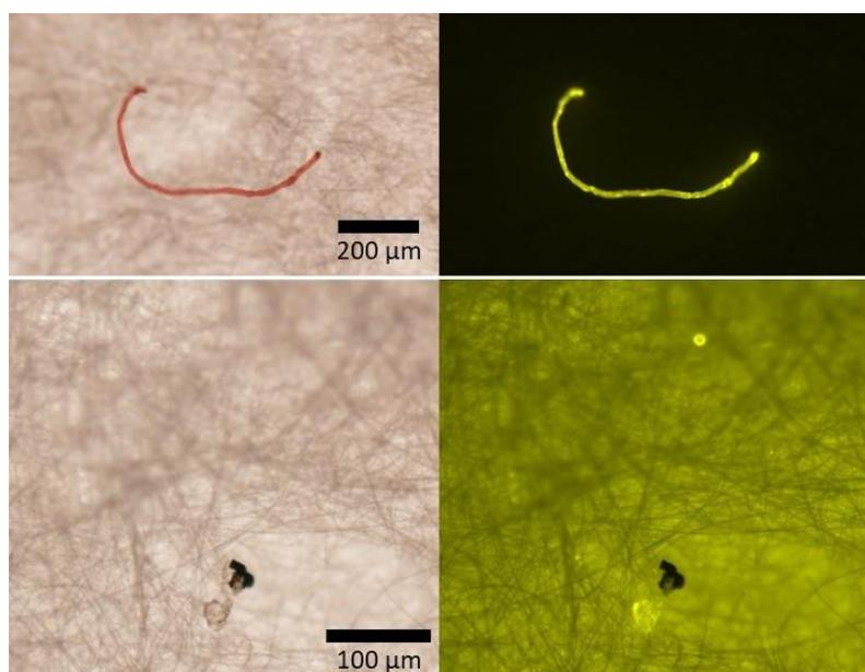
Figure 4. Examples of Nile red stained microplastics under ambient light (left) and blue light (455 nm) viewed with an orange filter (529 nm; right)
