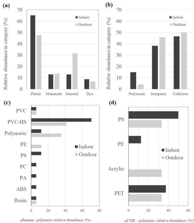
Figure 7. Abundance of different materials detected using  $\mu$ Raman (a) and  $\mu$ FT-IR (b), and relative abundance of the different polymeric materials detected using  $\mu$ Raman (c) and  $\mu$ FT-IR (d) in subsampled fragments and fibers. PVC=polyvinyl chloride, PVC-HS=polyvinyl chloride-heat stabilizer, PE=polyethylene, PS=polystyrene, PC=polycarbonate, PA=polyamide, ABS=acrylonitrile butadiene styrene, PET=polyethylene terephthalate.
