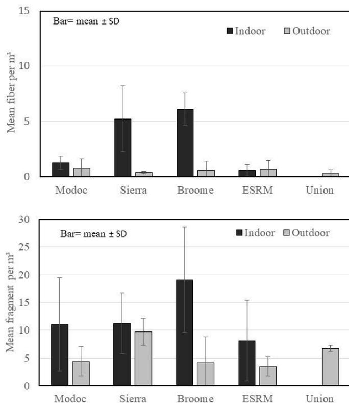
Figure 5. Microplastic fiber (top) and fragment (bottom) density per m<sup>3</sup> of air sampled across CSUCI from microscopy with Nile red. Bars: mean  $\pm$  1 SD.
