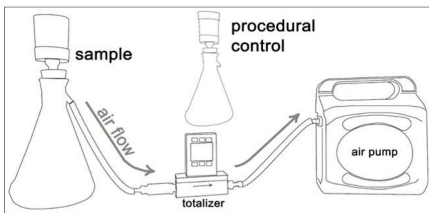
Figure 1. Vacuum filtration setup with filter, filter holder, GF filter (top left), vacuum flask (bottom left), airflow totalizer (middle), and vacuum pump (right). The procedural control was identical to the first elements, but not connected to a pump and with a cap added over the filter folder. This procedural control was placed adjacent to the sampling array.
