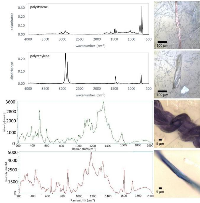
Figure 6. Representative images and spectra from μFT-IR (top two panels) and μRaman (bottom two panels).
